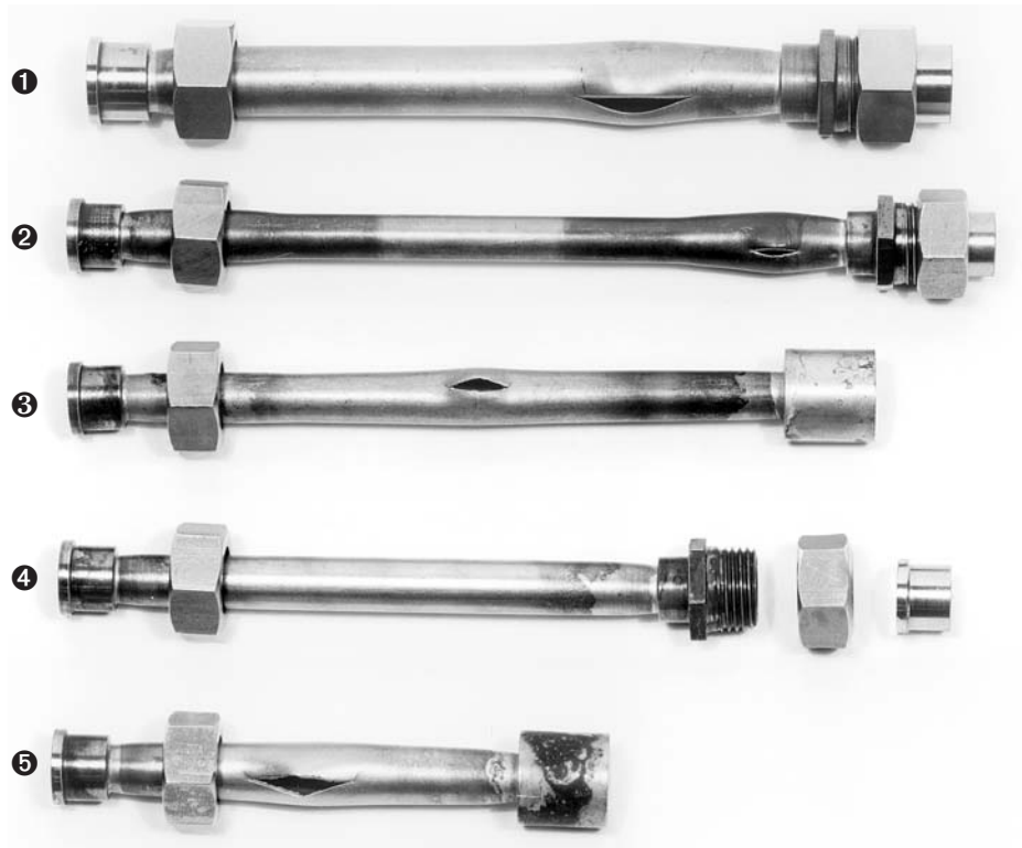
Mark VIII O-Seal tests demonstrate the reliability of brazed fittings.
