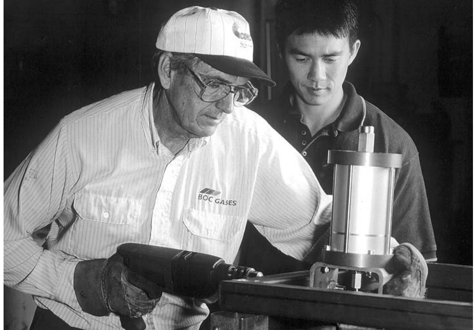
The new precision filling station at BOC Gases, Inc. in Chattanooga uses 12 air operated CPV FloMaster valves to fill mixed gases within 0.01% of spec.
