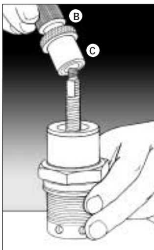
5. Invert items B and C with the "U" cup. Slip the tool assembly over the valve stem and into the bonnet gland.
