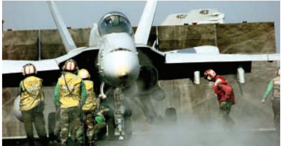
Flight deck personnel attach an F/A-18C "Hornet" to a catapult on board the nuclear powered aircraft carrier USS Roosevelt.
