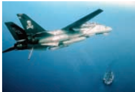
With tail hook down, a Fighter Squadron 84 (VF-84) F-14A Tomcat aircraft approaches for a landing aboard the aircraft carrier USS Roosevelt.
