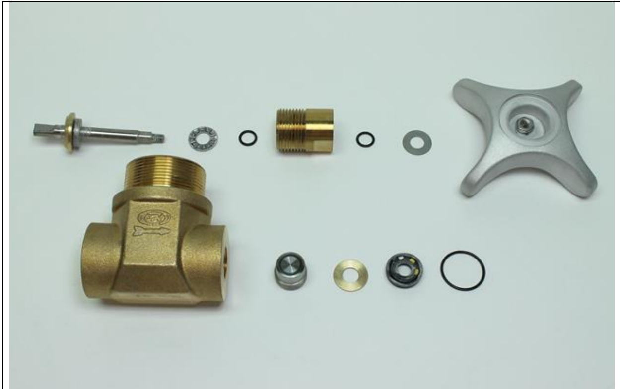
Photo 11: Post-test view of test article TA-1.5 after disassembly.
