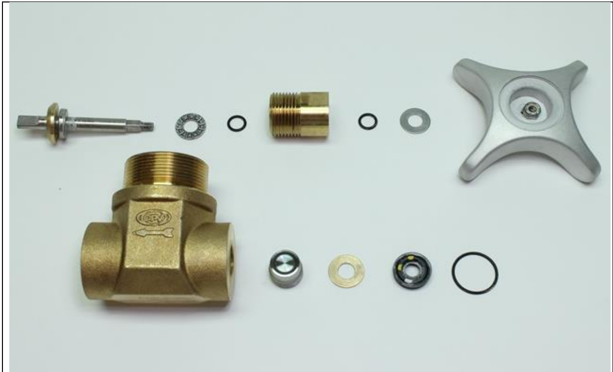
Photo 3: Post-test view of test article TA-1.1 after disassembly.
