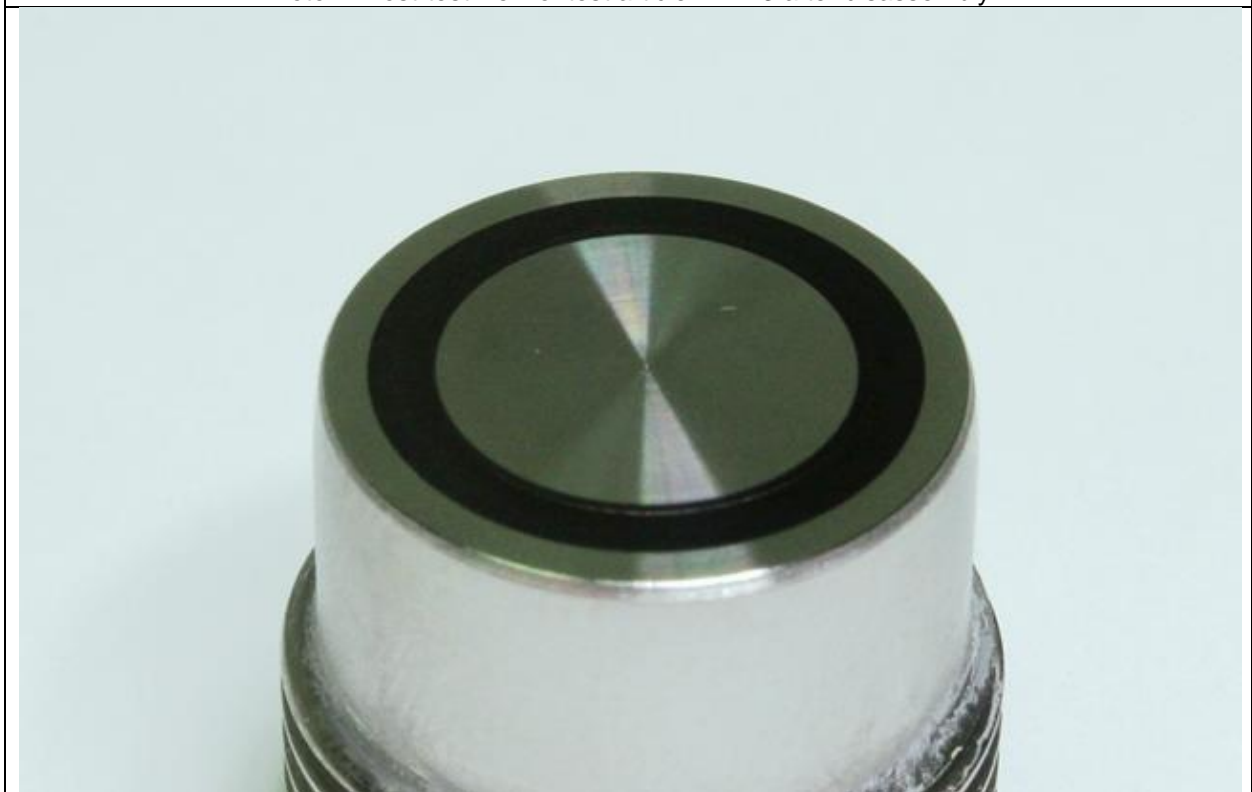
Photo 8: Post-test view of test article TA-1.3 shutoff valve seat.
