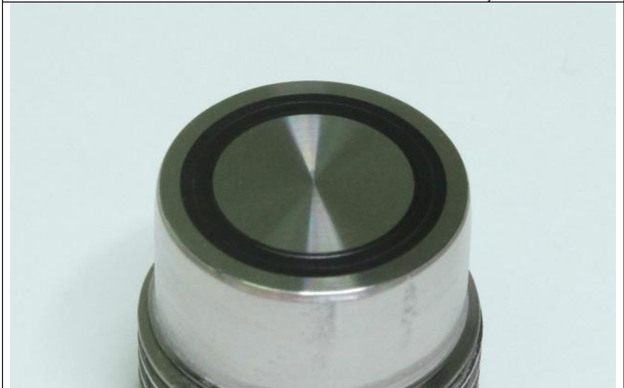
Photo 10: Post-test view of test article TA-1.4 shutoff valve seat.
