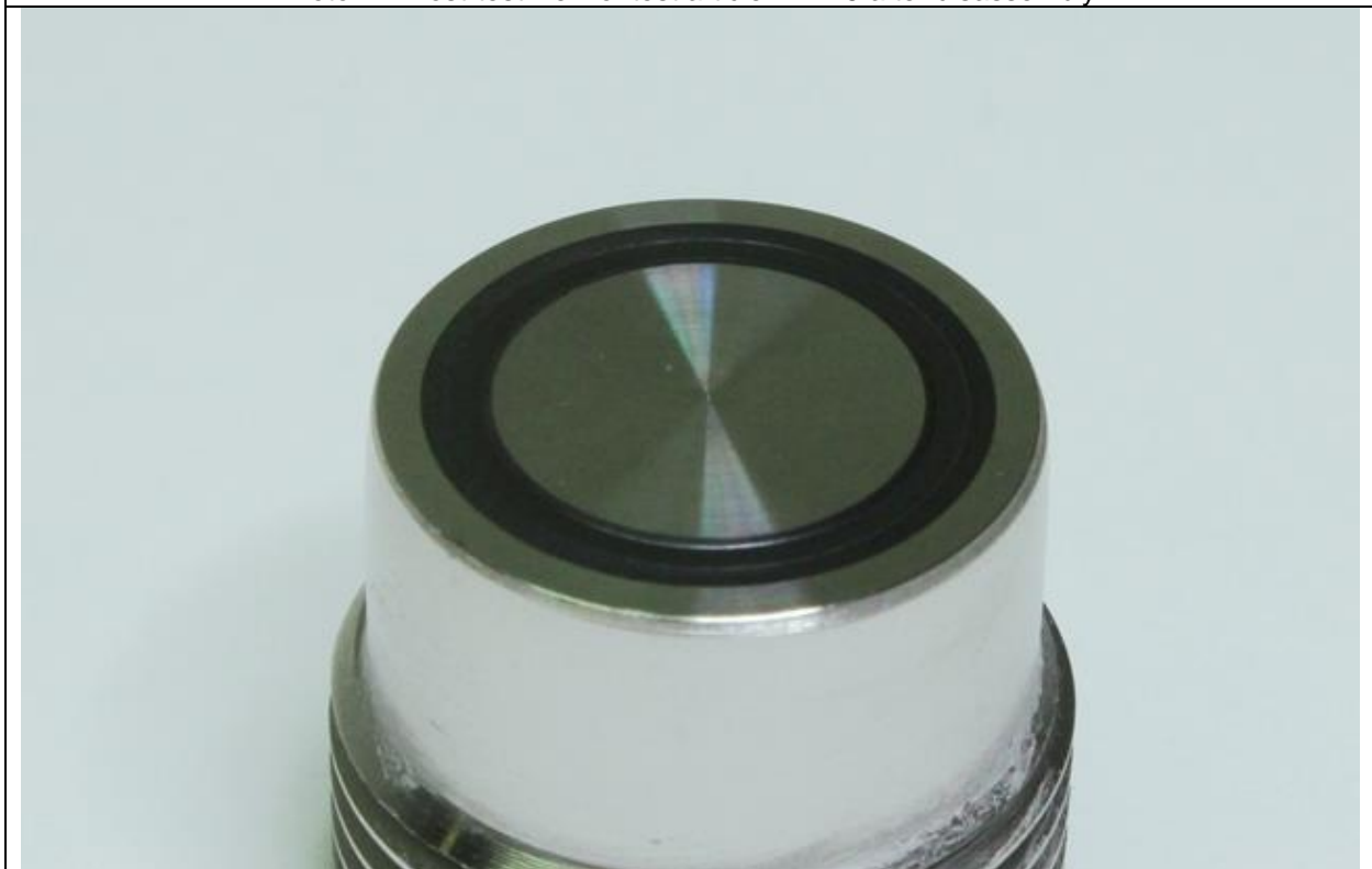
Photo 12: Post-test view of test article TA-1.5 shutoff valve seat.
