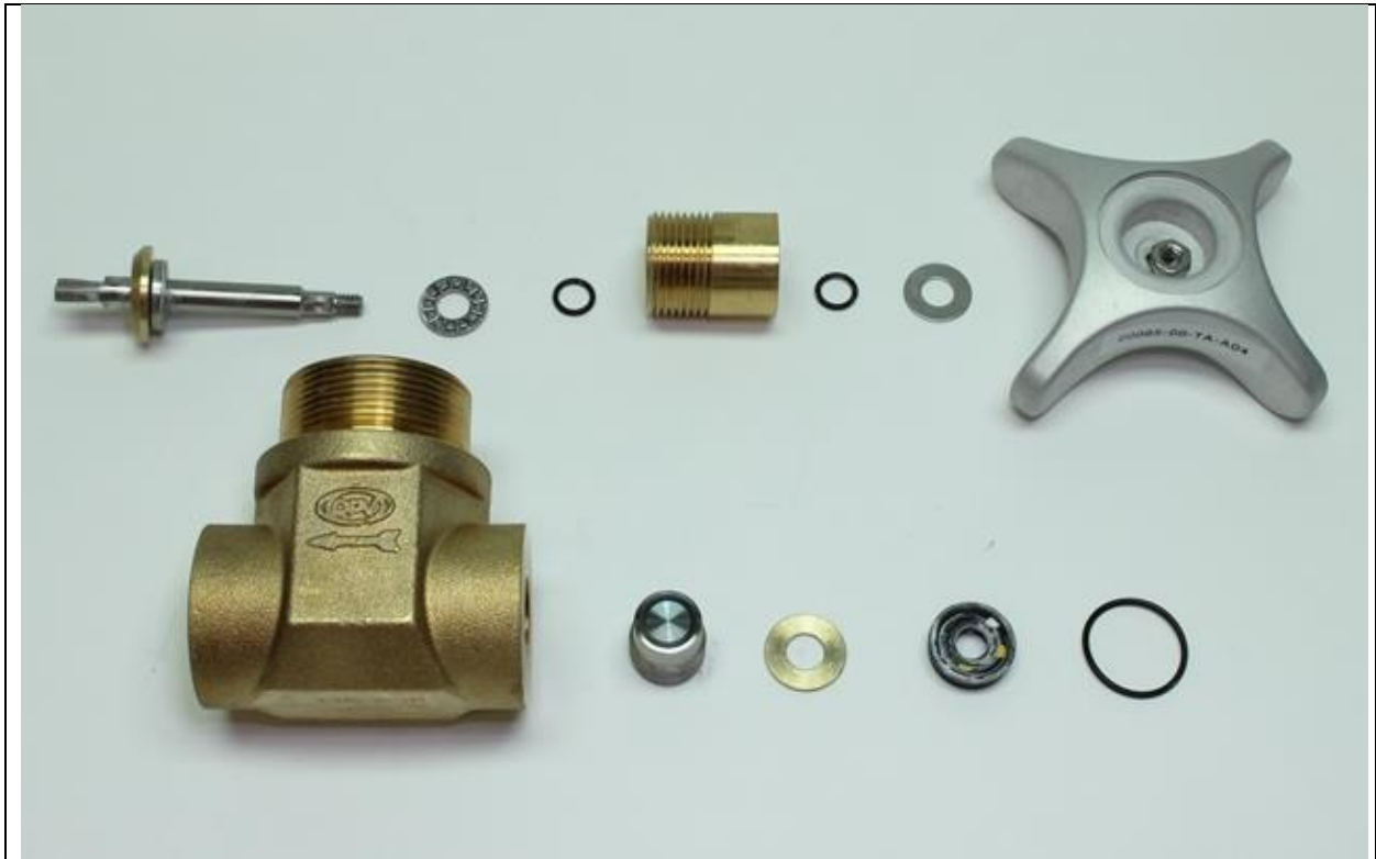
Photo 9: Post-test view of test article TA-1.4 after disassembly.
