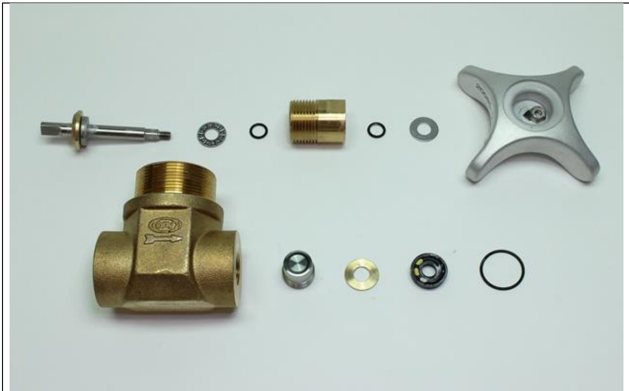
Photo 5: Post-test view of test article TA-1.2 after disassembly.
