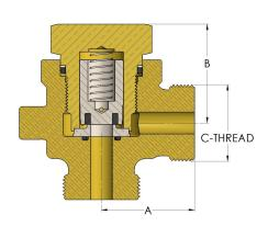
O-SEAL® Check Valves (600 Series) 1/4" Angle Check Valve with O-SEAL® Ends
