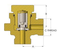
O-SEAL® Check Valves (600 Series) 1/2" Angle Check Valve with O-SEAL® Ends
